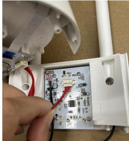
Step4: Use soldering iron to remove the wires from the board.
