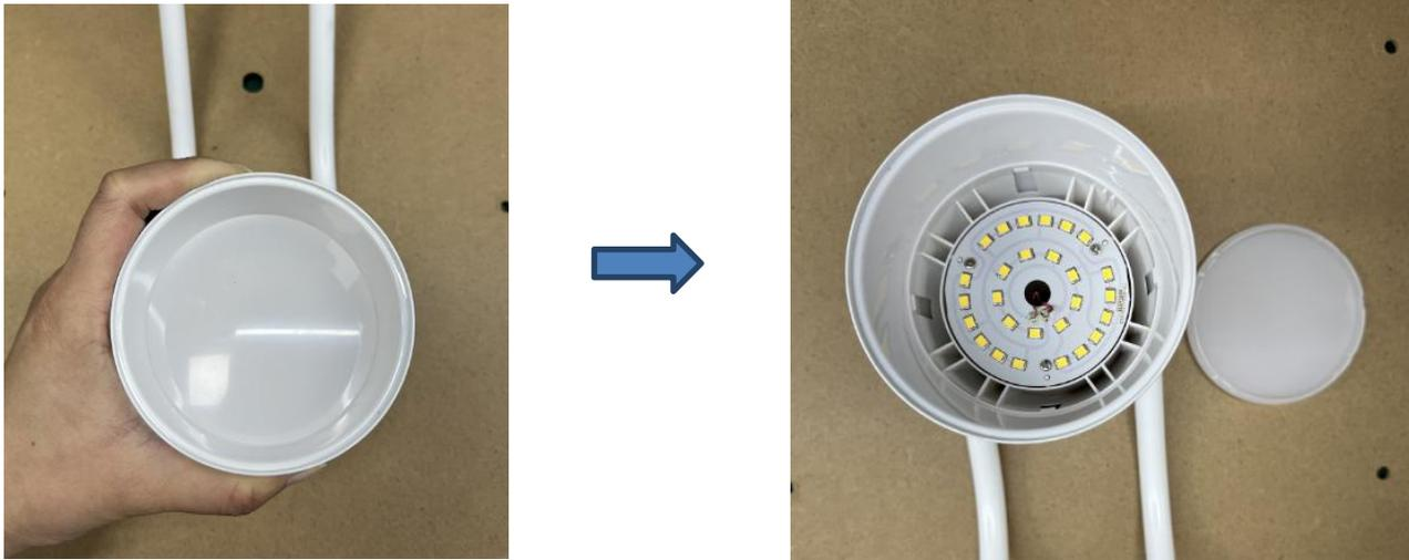
Step6: Use electric screwdriver to remove the screws on the light board, then pick up the light board with tweezers, and pull out the connection wire from the lamp pole.
