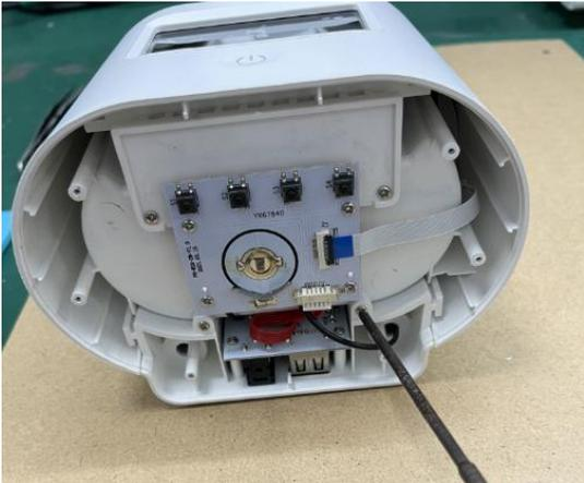
Step4: Slide the front plastic case up to expose the power board and remove the terminal of the cable.
