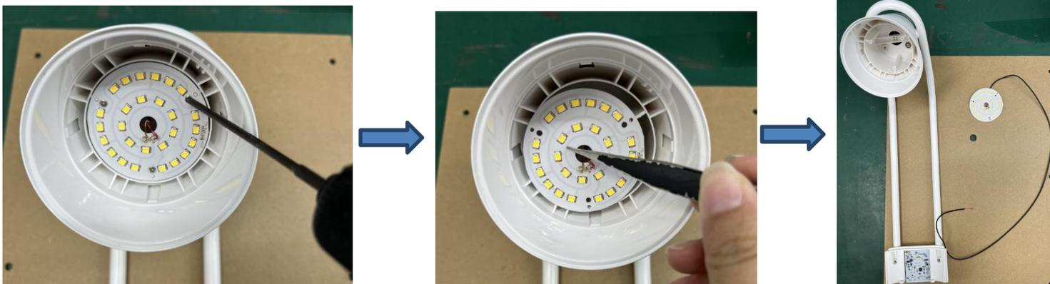
Step7: Now the light source was removed without being permanently damaged for verification purposes.
