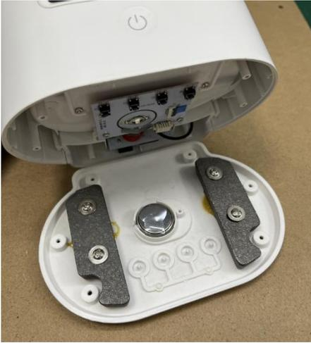
Step3: Remove the screws at the joint of the two parts of the plastic shell with electric screwdriver.
